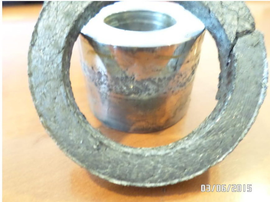
Sample Ring After Test Ring showed 50% adhesion
