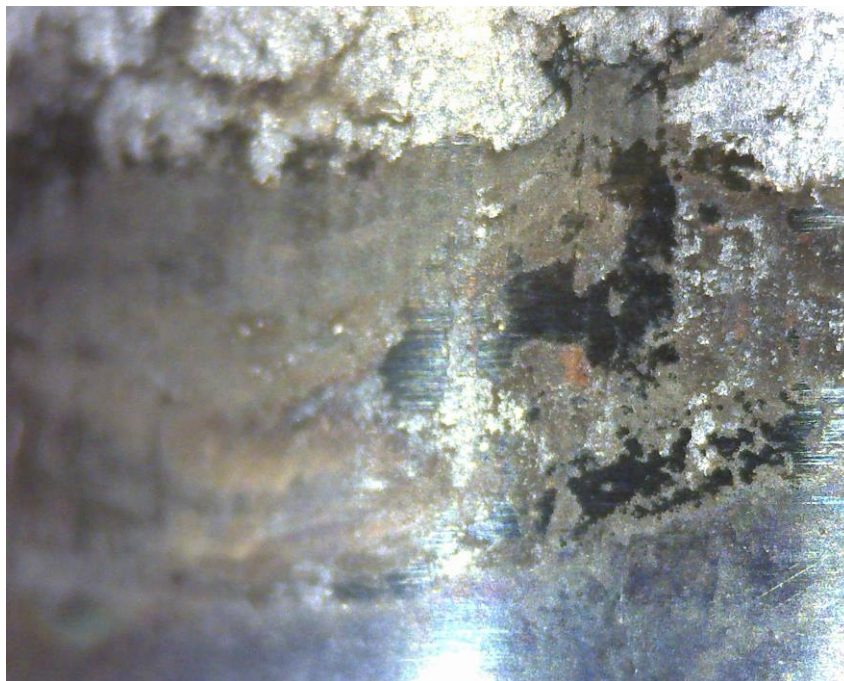
Cylinder surface in contact with packing ring (100X) <10% corrosion observed.
