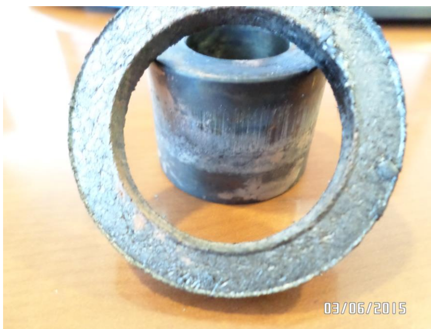
Packing ring and cylinder after test. 50% adhesion was observed.
