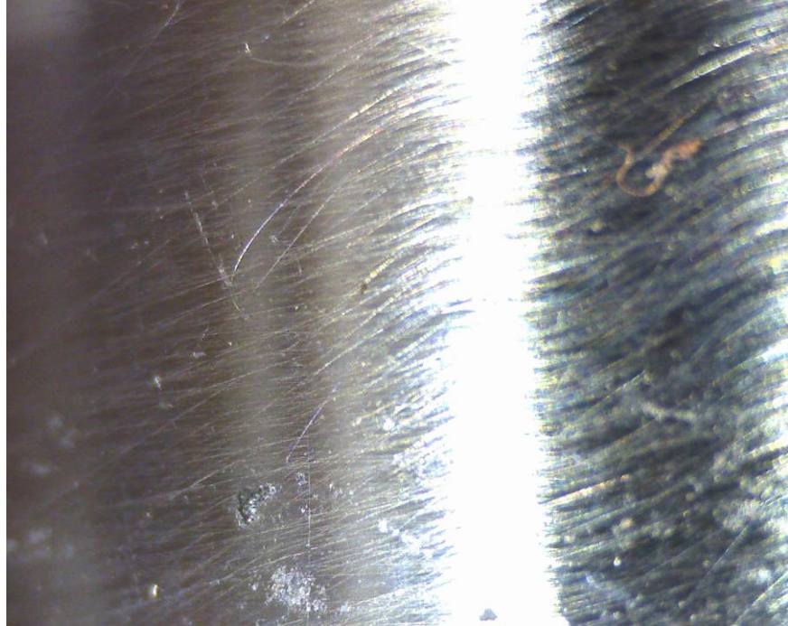
Cylinder surface in contact with packing ring (100X) <10% corrosion observed.
